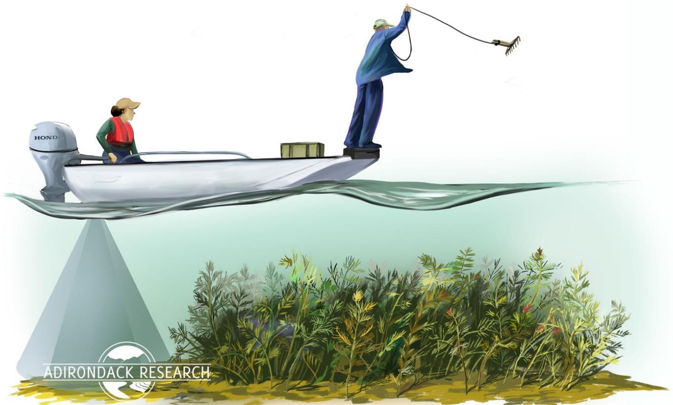
Figure 1: Illustration of the survey techniques utilizing a combination of sonar recording and manual rack toss.
